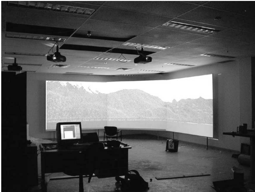
Fig. 2. The Immersion Lab at the Forest Sciences Centre, University of British Columbia, Vancouver, with three 8' × 10' screens in panoramic "wrap-around" configuration. (Credit: Duncan Cavens, Centre for Advanced Landscape Planning, UBC Faculty of Forestry).
