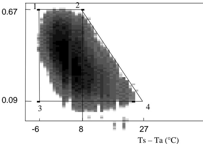
Figure 6:  $NDVI$  vs.  $Ts-Ta$  scattergram from Landsat TM images on Les Maures 90/08/09. Trapezoid vertices were estimated from scattergram using rules given above (From Vidal and Devaux-Ros, 1995).
