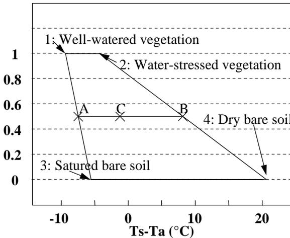
Figure 5: The theoretical trapezoidal shape showing the different biomass vs. water stress conditions of a canopy-soil continuum (from Moran et al., 1994). The WDI (water deficit index) of point C is given by AC/AB as shown in Equation 8.
