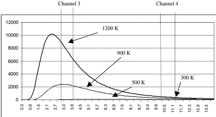
Figure 1: Plank radiances for blackbody temperatures from 300 K to 800 K. Temperature increases are greater under channel 3 than under channel 4
