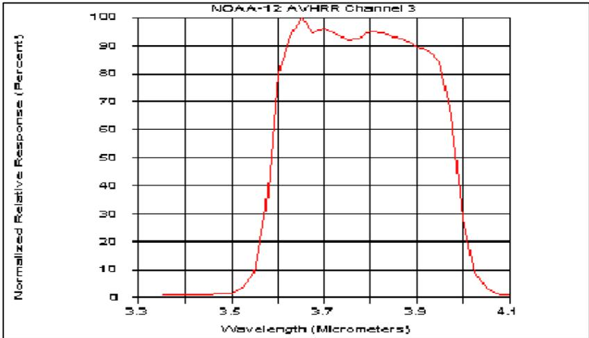
Figure 2: Normalised spectral response of Channel 3, AVHRR-NOAA 12
