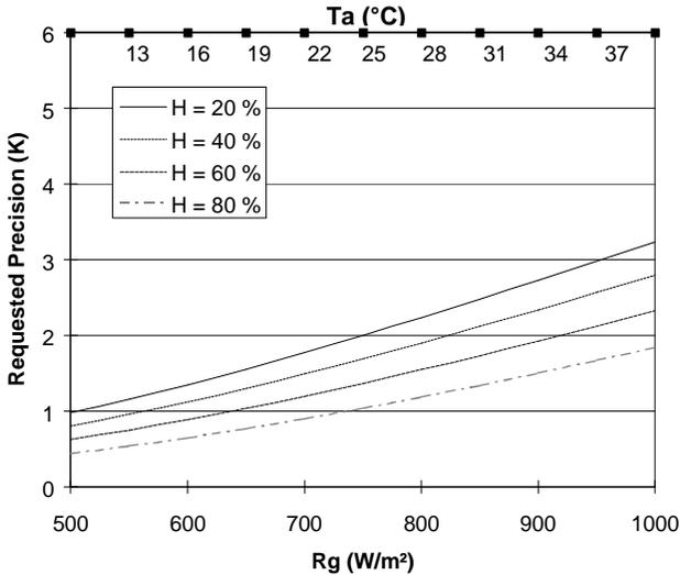
Figure 2: Requested precision for vegetation stress estimation on forest ( $r_a = 16$  s/m) as a function of global radiation  $R_g$ , air temperature  $T_a$  and air moisture (from Vidal et al., 1997)
