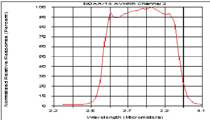
Figure 3: Normalised spectral response of Channel 3, AVHRR, NOAA 14.
