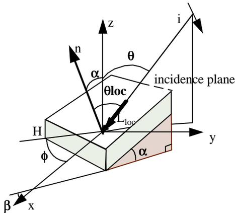
Figure 6: Scattering geometry over hilly terrain
